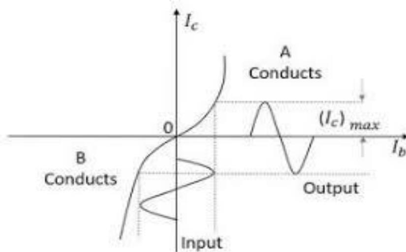
**Fig: Waveforms of output current and voltage**
