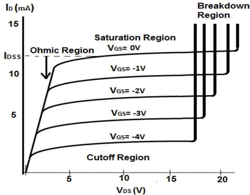
**Fig: Drain characteristics curve**
