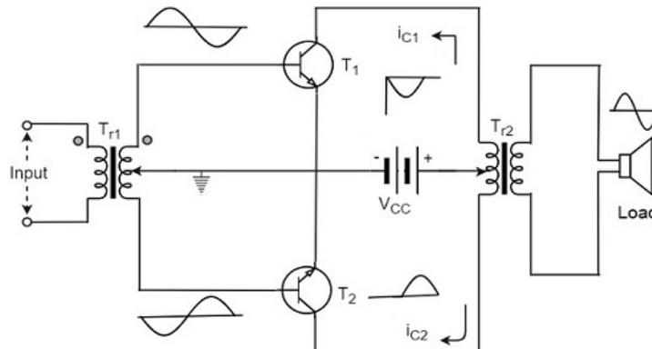
**Fig: Class B push pull amplifier**
