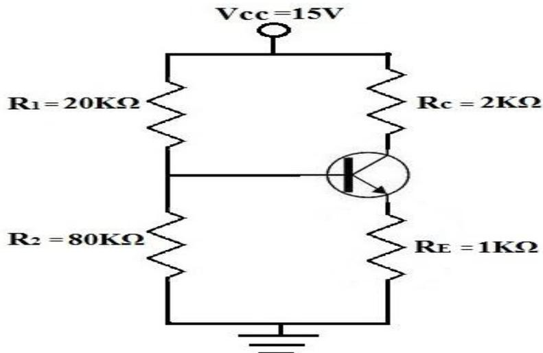
Fig: Voltage Divider Bias Circuit
