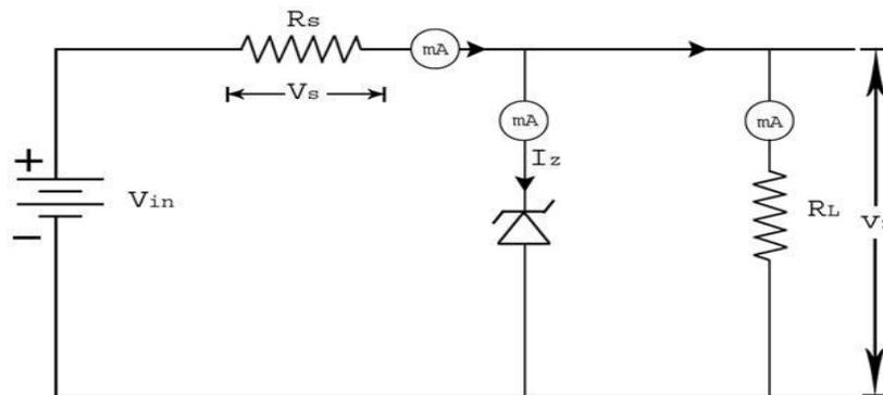
Fig: Zener diode as voltage regulator
