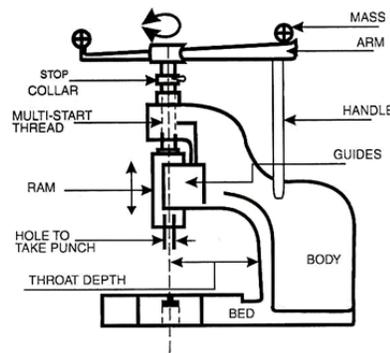
Fig. A manually operated (Fly) Press.
