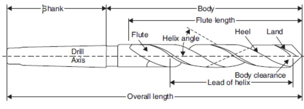
Fig Nomenclature of a standard twist drill
