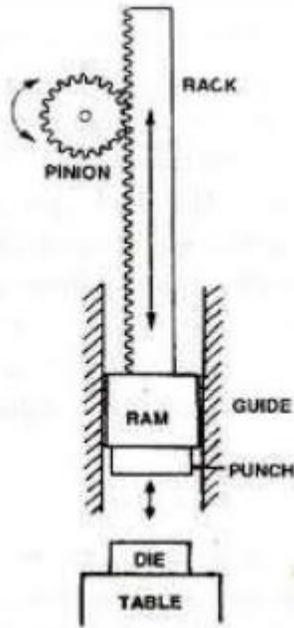
Fig. 5.48 Press Forging
