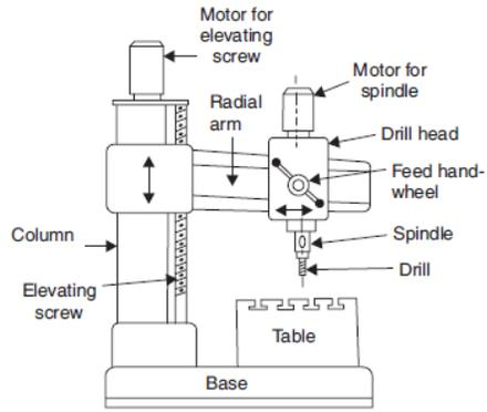
Fig. Radial drilling machine
