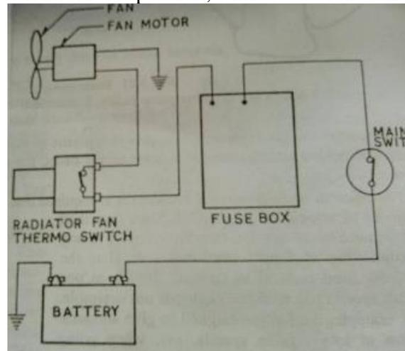
**Figure: Electrically Driven Fan Circuit**
