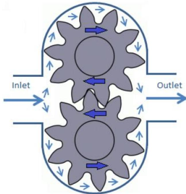
**Figure: Externally Mesh Gear Type Pump.**
