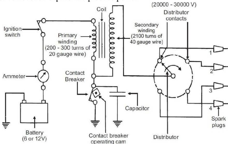
**Figure: Battery Ignition System**
