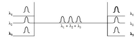
Fig: Wavelength-Division Multiplexing
