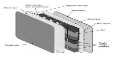
Working of Plasma display: When a voltage is applied, the electrodes get charged and cause the ionization of the gas resulting in plasma. This also includes the collision between the ions and electrons resulting in the emission of photon light.
