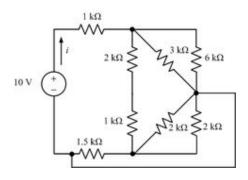
d. Find the current in  $10 \Omega$  by using superposition theorem.
