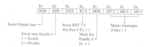
SOD – Serial Output Data: Bit D7 of the accumulator is latched into the SOD output line and made available to a serial peripheral if bit D6=1;
