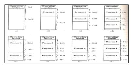
Total memory size is 64M.from this 8M partition is occupied by operating system and remaining can be partitioned as per the size of the process
