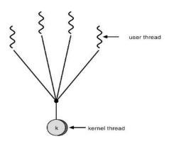
**2. One-to-One:** It maps each user level thread to a kernel level thread. Even one thread makes a blocking call; other thread can run with the kernel thread.
