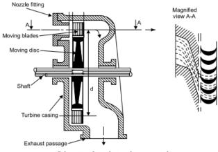
Schematic of simple impulse steam turbine stage
