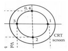
iii) the phase difference between the two sinusoidal signals by using formulae, when the Lissajous figures are of **elliptical shape**
