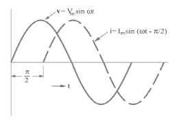
For pure inductive circuit, current 'i' lags behind applied voltage 'v' by 90<sup>0</sup> ( or  $\pi/2$ )rad
