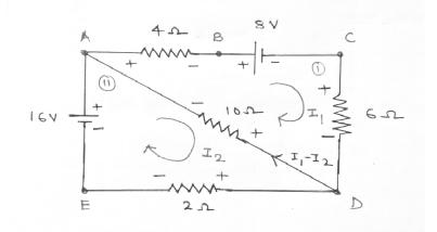
Apply KVL to loop (I) – (A-B-C-D-A) -4 I<sub>1</sub> -8-6I<sub>1</sub>-10(I<sub>1</sub>-I<sub>2</sub>) = 0 -4I<sub>1</sub>-8-6I<sub>1</sub>-10I<sub>1</sub>+10I<sub>2</sub> = 0 -20I<sub>1</sub>+10I<sub>2</sub> = 8 -10I<sub>1</sub>+5I<sub>2</sub> = 4.....(1)
