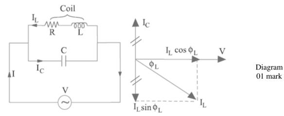
We will consider the practical case of a coil in parallel with a capacitor, as shown in above fig. Such a circuit is said to be in electrical resonance when the reactive component of line current becomes zero. The frequency at which this happens is known as resonance frequency.
