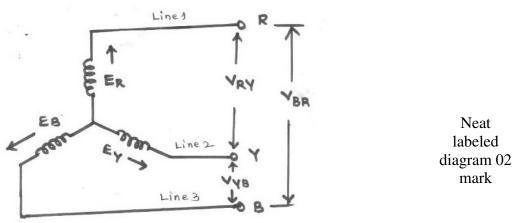
As seen from the above diagram, in this form of interconnection, there are two phase windings between each pair of terminals but since there similar ends have joined together, they are in opposition.
