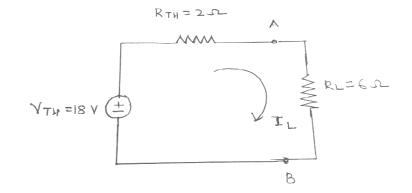
$$I_L = \frac{V_{TH}}{R_{TH} + R_L} = \frac{18}{2+6} = 2.25 A.$$
