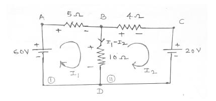
Apply KVL for loop I- (A-B-D-A)  $-5 I_1 - 10 (I_1 - I_2) + 60 = 0$   $-5 I_1 - 10 I_1 + 10 I_2 = -60$   $-15 I_1 + 10 I_2 = -60$   $-3 I_1 + 2 I_2 = -12$ -----equation (1) 01 mark
