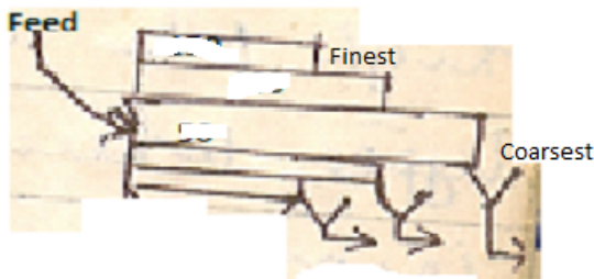
d) Different size screen on concentric trommels.
