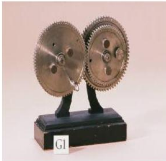
Fig- Compound Gear train
