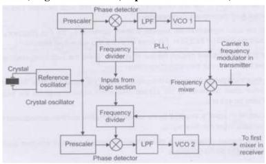
The synthesizer is used for developing all the signals used by the transmitter and receiver.
