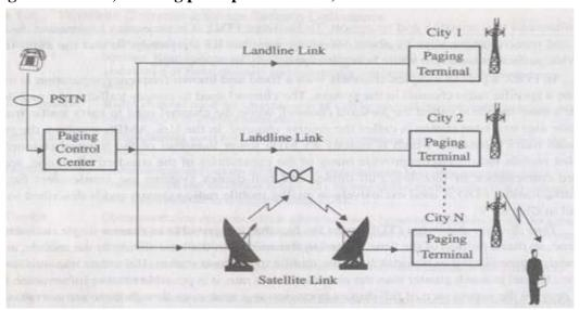
Pager is a Simplex Communication Device. Paging Systems are communication systems that send messages to a subscriber. Message can be numeric or alphanumeric. Paging Systems are used to notify a subscriber of the need to call a particular telephone number or to travel to a location to receive further instructions. In modern paging systems, news headlines, faxes can also be sent.
