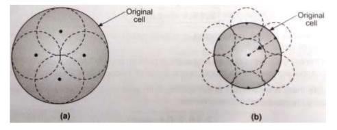
Let every cell have radius reduced to half. The new base stations are therefore needed in the region to increase the number of channels in the area to reduce the area served by a single base station.
