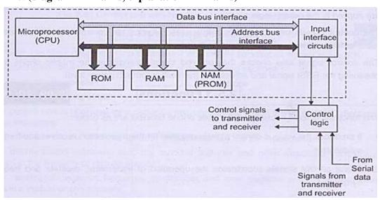
The logical unit contains the main control circuitry for the cellphone unit. The logical unit consists of a CPU, RAM, ROM, I/O interface circuit and control logic. NAM (Number Assignment Module) is a programmable read only memory (PROM). The NAM holds the Mobile Identification Number (MIN) i.e. the telephone number of the mobile phone.
